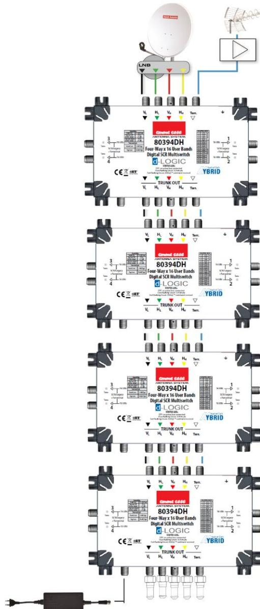
All 4 LNB trunks should always be cascaded or terminated with a DC-blocked 75-Ohm terminator. All unused SCR/Legacy outputs should be terminated with a 75-Ohm terminator for proper terrestrial signals.
